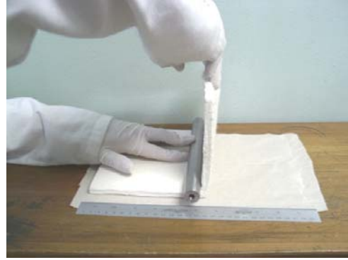
Fig. 5. Compressive test and flexibility of thermal insulator blankets
