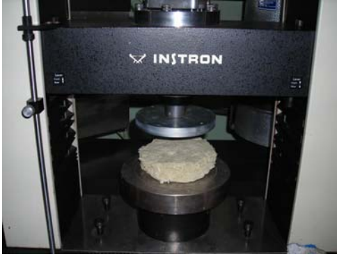
Fig. 5. Compressive test and flexibility of thermal insulator blankets
